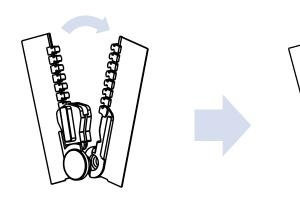
Completely new and easy way to close the zipper. Simply position and snap open parts. Open parts components automatically rotate and engage by pushing open parts down. Components are enlarged for easier hand assembly/operation.
